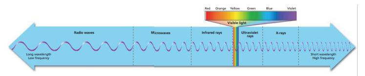
The **electromagnetic spectrum** is the complete range of electromagnetic waves placed in order of increasing frequency. **The electromagnetic spectrum is made up of radio waves, infrared rays, visible light, ultraviolet rays, X-rays, and gamma rays.**
