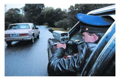
distance. To measure speed, a radar device uses the Doppler effect. Because the car is moving, the frequency of the reflected waves is different from the frequency of the original waves. The difference in frequency is used to calculate the car's speed.
